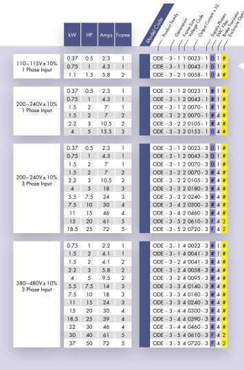
Replace # in model code with colour-coded option **Enclosure Types** Outdoor Use Non-switched В **Outdoor Use EMC** Filter Internal EMC Filter F
